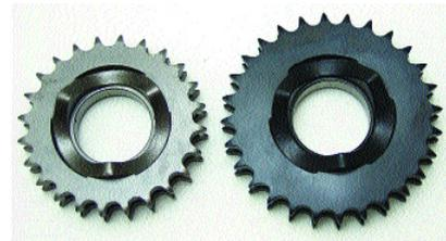
The sprocket on the left is the stock 24-tooth unit and the one on the right is the new 28-tooth sprocket from Baker.
