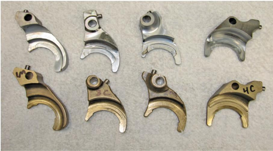
That added amount of slop in the system, hinders the ability to hold gears in place, as well as eliminating the smooth nature of sliding gears up and down the shaft splines that you as a rider are after. The Baker fork tines had an overall fitment gap of .007" to .011" throughout the 4 forks. Tighter is better, no secret to all of us, wink, wink, and the better fitting your forks are, the faster and more firmly they will move gears into place when the transmission is shifted.
