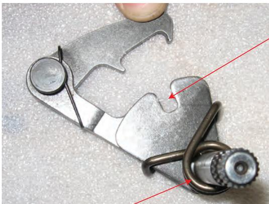
Shifter pawl adjustment set screw landing spot interacts with steel pawl plate then the spring. Pawl plate has to slide against the pawl lever body on every shift. Added friction kills smooth shift feel.
