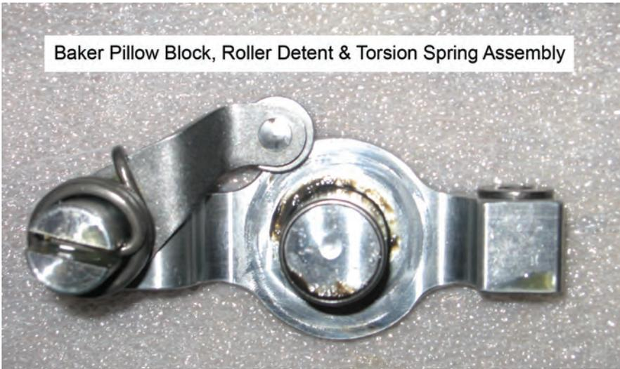
Roadmax Pillow Block, Roller Detent, & Torsion Spring Assembly
