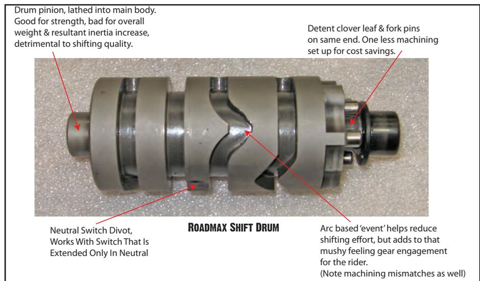
block mounting system all play a part. The drum track design in it's most basic form is dictated by the amount that you want to throw each gear, the angle of the tracks in and out of gear (the 'event'
