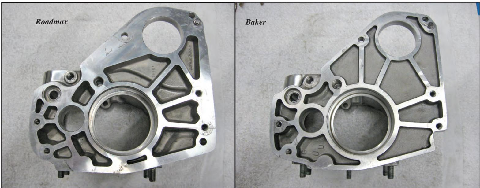
like a cube, the top and bottom, left and right surfaces are parallel and perpendicular to each other, respectively. The ability to hold these dimensions accurately directly affects the relationship of the gearset and the shift system, the gearset and the clutch and the alignment of the entire drivetrain. Both units' surfaces were within what I feel to be allowable limits, on a parallel and perpendicular nature, less than  $.1^\circ$  total variance (about .010") throughout.
