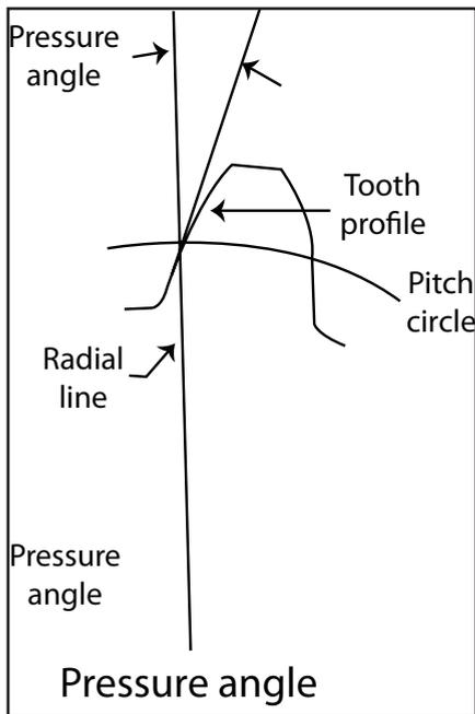
the intended tooth profile to be straight across the contact face. (Some high horsepower applications utilize crowned teeth to compensate for deflection enabling flat tooth contact under full load, rather than edge only loading when the middle of the tooth deflects.)
