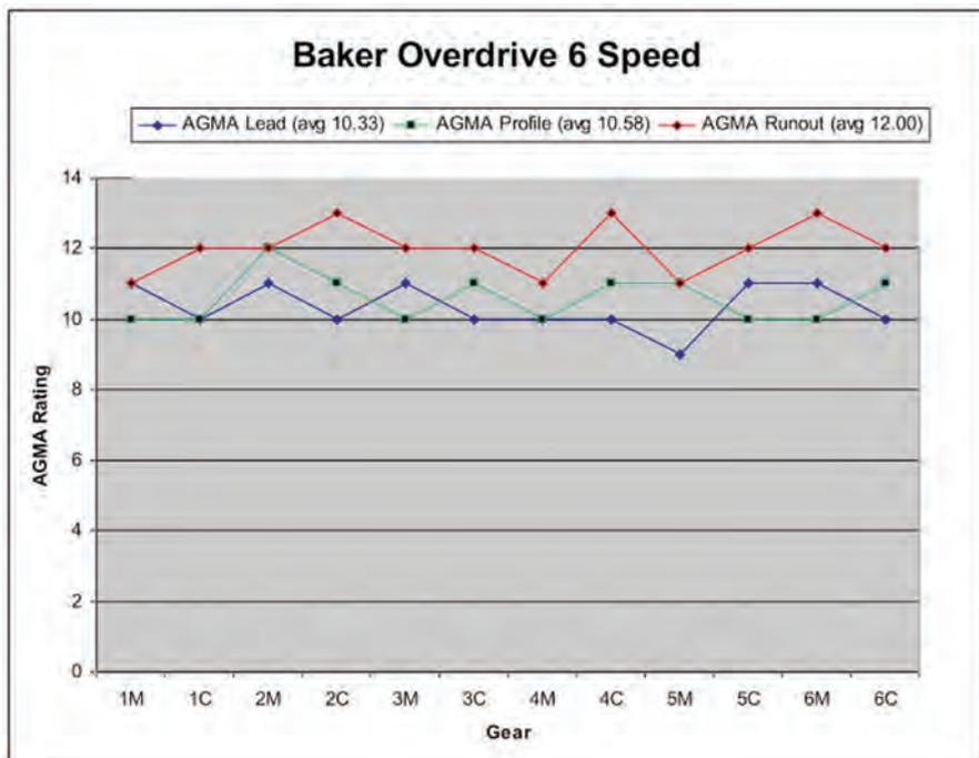
bearing journals, but incurred greatly different results for spline runout. The Roadmax unit had a total indicated spline runout of .0039" vs. the .0014" for the Baker. The Countershaft was basically the same story, Roadmax .0022" and the Baker came in at .0010". Once again, control of the manufacturing process was the difference.
