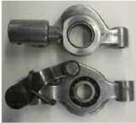
The shift drum has a spring-loaded detent that holds it in gear each time the drum is moved. Here are a 1979-99 plunger detent (top) and a 2000 and later roller detent.
