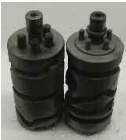
**The pawl pins on the end of a 1979-99 drum (left) are 1/4" thick and 4mm on 2000 and later versions. The number of pawl pins also changed in 2000, going from four to five.**
