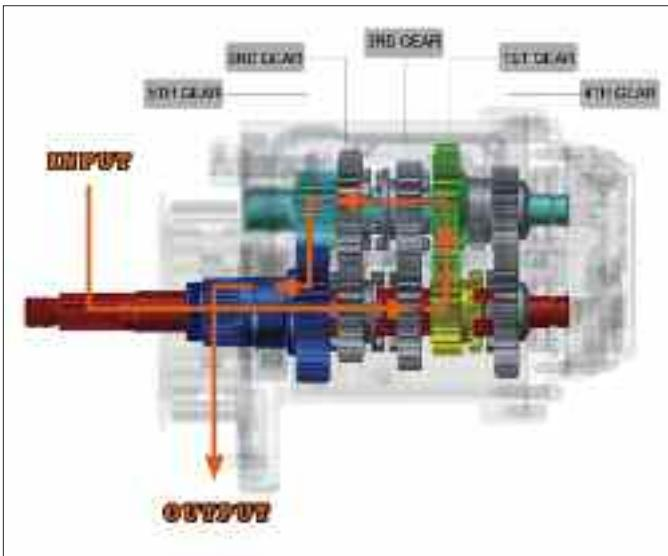
This illustration shows how power flows into, through, and out of the transmission when it's in first gear.
