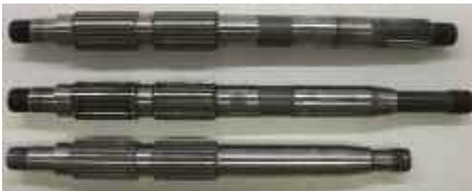
Here are three of the four types of mainshafts used in a five-speed (bottom to top), from mid-1979 to early-1984, from mid-1984 to 1989, and from 1991 to 2006.
