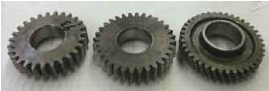
From left to right, an early stub tooth gear, a high-contact ratio gear, and a Cruise Drive six-speed helical gear.
