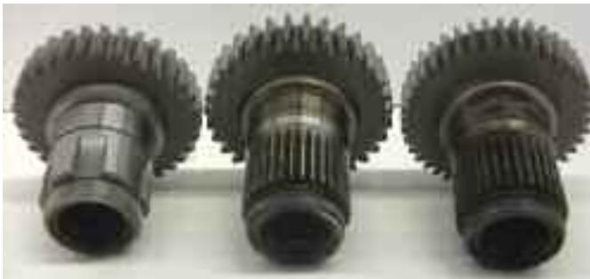
Here are three of the four types of main drive gears used (left to right): from 1979 to early-1984, from 1991 to 1993, and from 1994 to 2006.
