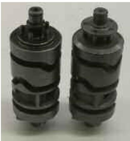
**A shift drum with unsupported 4mm pawl pins is on the left; a supported drum is on the right.**
